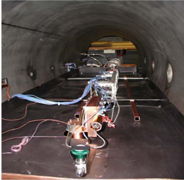
Figure 9. Hydrogen CLHP in Thermal Vacuum Chamber
