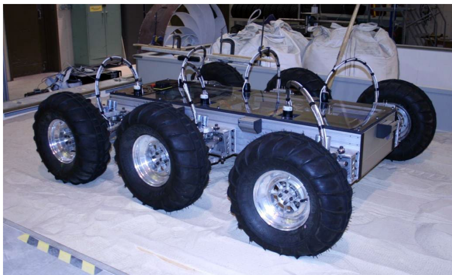
Figure 19.—Glenn’s dedicated tire test vehicle, Proteus, which was developed to simulate various driving configurations.
