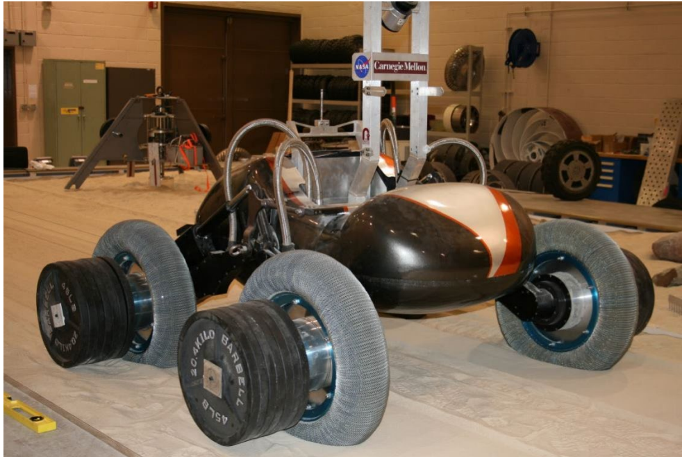
Figure 18.—Scarab rover (Wettergreen et al., 2010), one of the vehicles used for drawbar pull (DP) testing at NASA Glenn Research Center.
