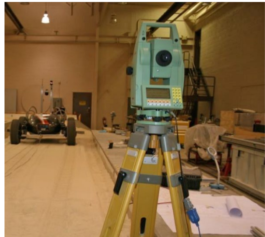
Figure 28.—Robotic laser tracking system used to measure vehicle velocity.
