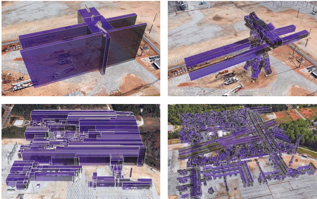
Figure 7. Variations of obstacle field size and detail to test ICAROUS capacity. Top left: 500 kV Section, 2.5 D representation. Top right: 500 kV Section, 3D representation. Bottom left: North Quarter, 2.5 D representation. Bottom right: North Quarter, 3D representation. © Lidar data: Southern Company; Map data: Google & DigitalGlobe
