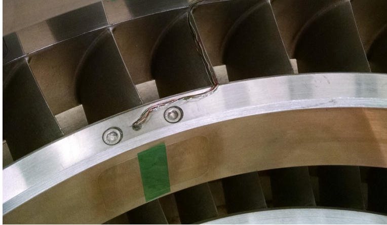
Figure 2.14: Photograph of wire routing on upstream face of hub shroud and along leading edge of adjacent stator vane to wire egress hole in casing. Clean-release protective tape shown here covering the sensors from damage was removed prior to operation.
