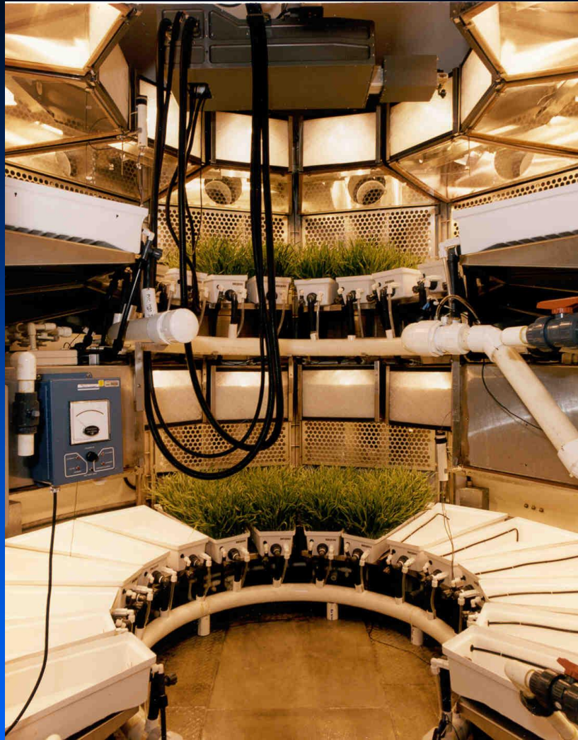
ALSARM Robot in NASA Biomass Production Chamber
