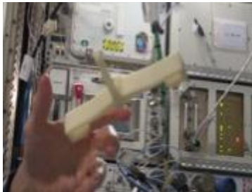
SPHERES Tow Hitch: SPHERES consists of 3 free-flying satellites on-board ISS. Tow hitch joins two of the SPHERES satellites together during flight. Printed 2/21/17.
