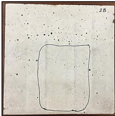
Martian simulant JSC Mars-1A, stucco mix, Portland cement, and water
