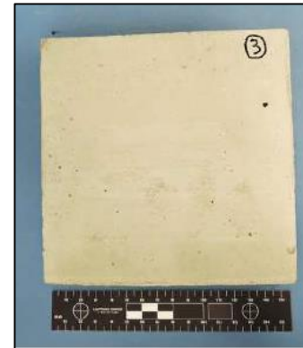
Lunar simulant JSC-1A, stucco mix, Portland cement, and water
