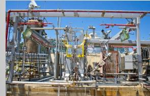
SpaceX subscale component for Raptor methane-fueled engine
