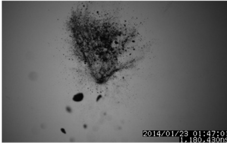
Figure 7.—Ice particle impact. The impact was captured with the Shimadzu camera and used to measure the fragments equivalent diameter distribution presented in Figure 6 (Ref. 28).
