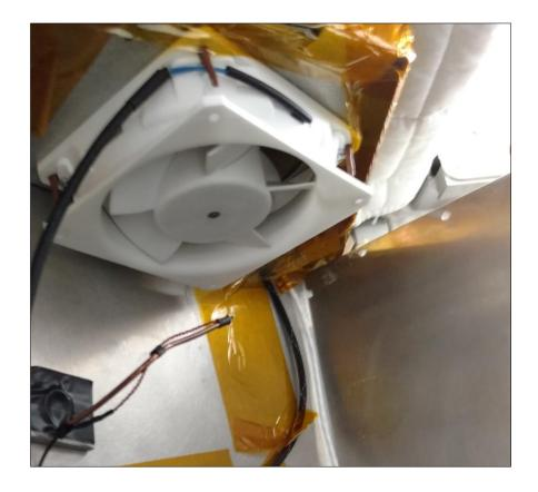
Movement of fan blade tips via embedded magnets produce the noise cancelation signal →
