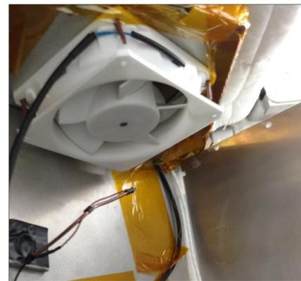
Movement of fan blade tips via embedded magnets produce the noise cancelation signal →
