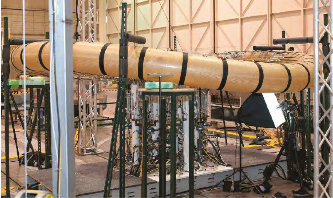
Figure 43. Out-of-plane buckling (test run #1 / T5C-1 / 20 psi / compression).
