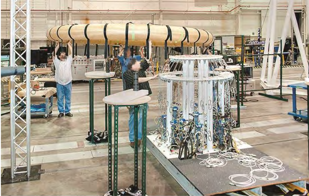
Figure 38. Flight Loads Laboratory technicians placing the test article in the test setup.
