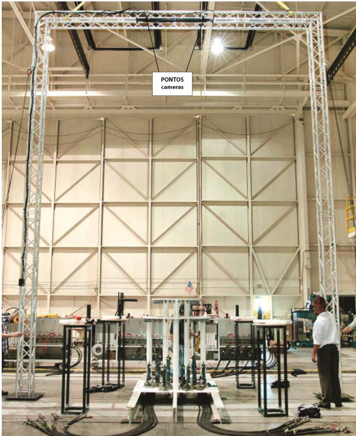
Figure 28. The setup of the PONTOS cameras.
