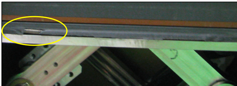
Figure 4. Sliding seals can lead to wear and tear thus allowing gas and vacuum leaks around the ram skirt.
