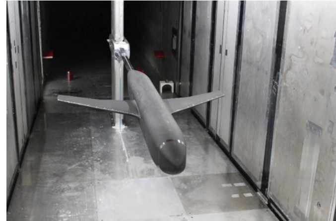
2.5% Juncture Flow Model in the VA Tech 6-foot Stability Wind Tunnel Aug 2015
