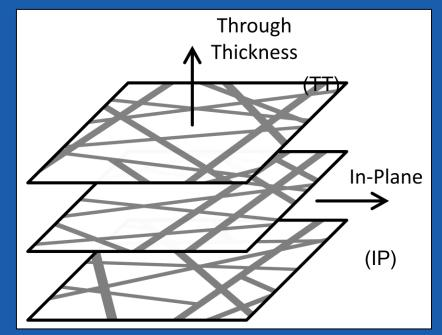
Schematic of a Transverse Isotropic Material
