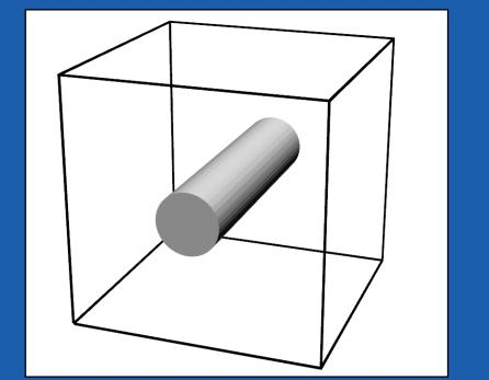
Simulated Domain for Square Array of Cylinders
