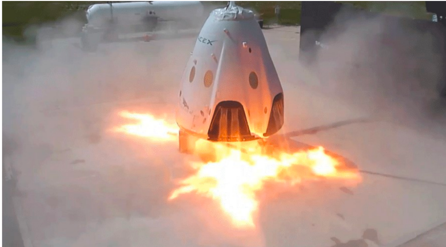
SuperDraco thrusters on SpaceX's Dragon 2 spacecraft 1
