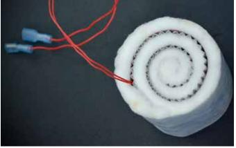
Lab Prototype of the Capacitor
