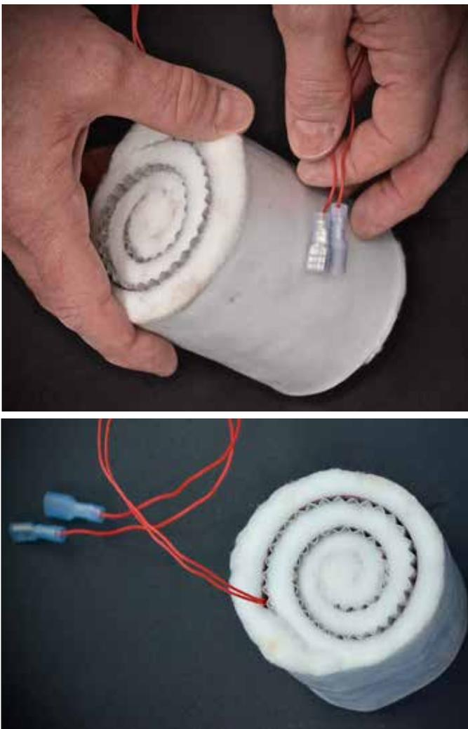
Lab Prototype of the Capacitor
