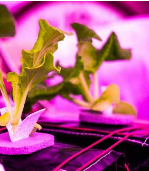
which environmental variables (e.g. temperature, relative humidity, light intensity) can be tracked and controlled in support of whole plant physiological testing (up to 135 days) and Bio-regenerative Life Support System (BLSS) investigations. The BLSS approach capitalizes on the ability of plants to produce oxygen,
