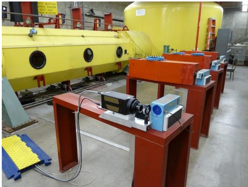
Fig. 11. HFFAF test section and a PI-MAX shadowgraph camera station, looking northeast. The camera, imaging lens and Kerr cell assembly without the Kerr cell are visible.
