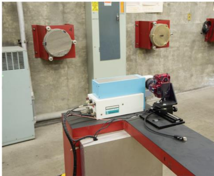
Fig. 15. A Nikon shadowgraph camera station, looking south. The camera and the Kerr cell assembly are visible in the foreground. The imaging lens is sandwiched in between the Kerr cell and the camera. The focusing mirror is in the background.
