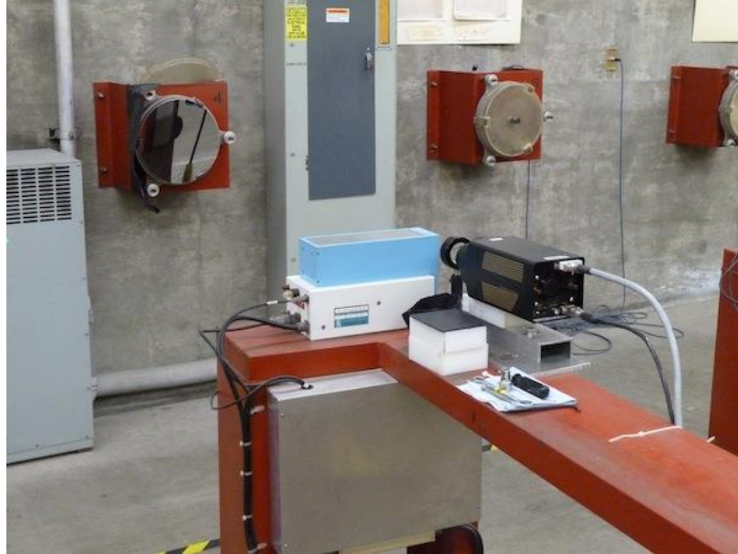
Fig. 12. A PI-MAX shadowgraph camera station, looking south. The camera, imaging lens and Kerr cell assembly without the Kerr cell are visible in foreground. The focusing mirror is in the background.
