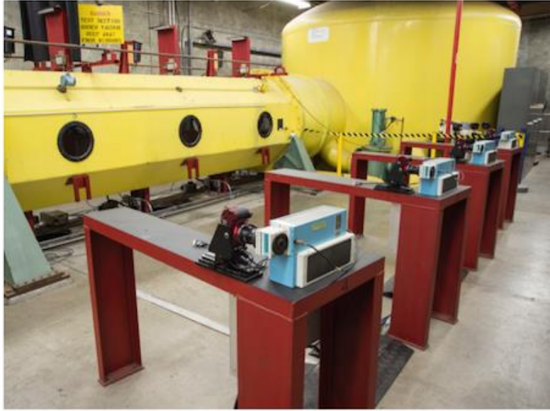
Fig. 14. HFFAF test section and a Nikon shadowgraph camera station, looking northeast. The camera and Kerr cell assembly are visible. The imaging lens is just to the left of the Kerr cell.
