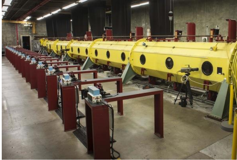
Fig. 16. HFFAF test section and Nikon shadowgraph camera stations, looking west. This photo corresponds to Fig. 1, which shows the original horizontal sheet film shadowgraph stations.
