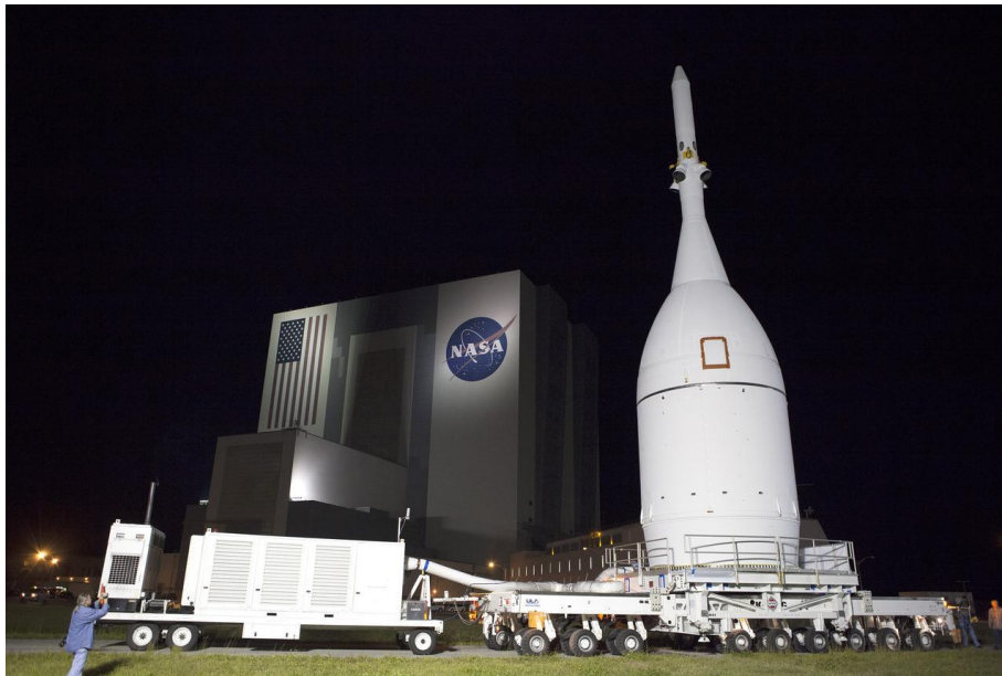
Figure 5. Orion/SM/LAS transporter from LASF to VAB. MPPU on the left. 4
