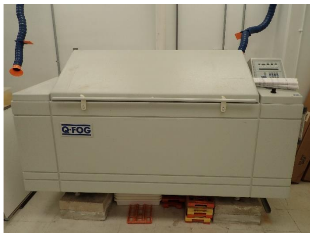
Figure 1. Q-Fog programmable CCT-1100 cyclic corrosion salt fog chamber.
