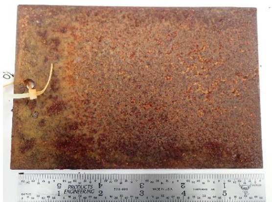
Figure 5. 1018 Carbon steel calibration panel following 119 days of atmospheric exposure.
