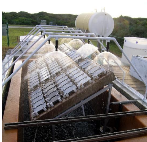
Figure 2. Alternating Seawater Spray Test apparatus.
