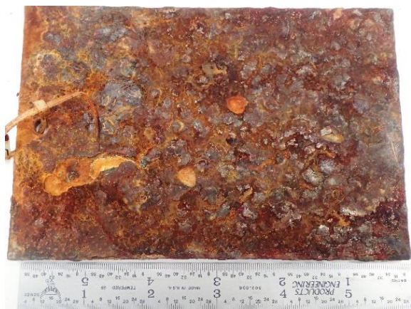
Figure 3. 1018 Carbon steel calibration panel following 97 days of ASST exposure.
