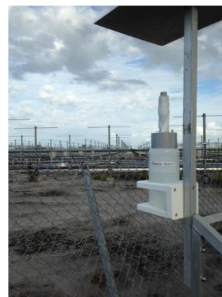
Figure 7. Chloride concentration collection candle wick located at the Ascent Wind Profiler site near the Shuttle Landing Facility (SLF).
