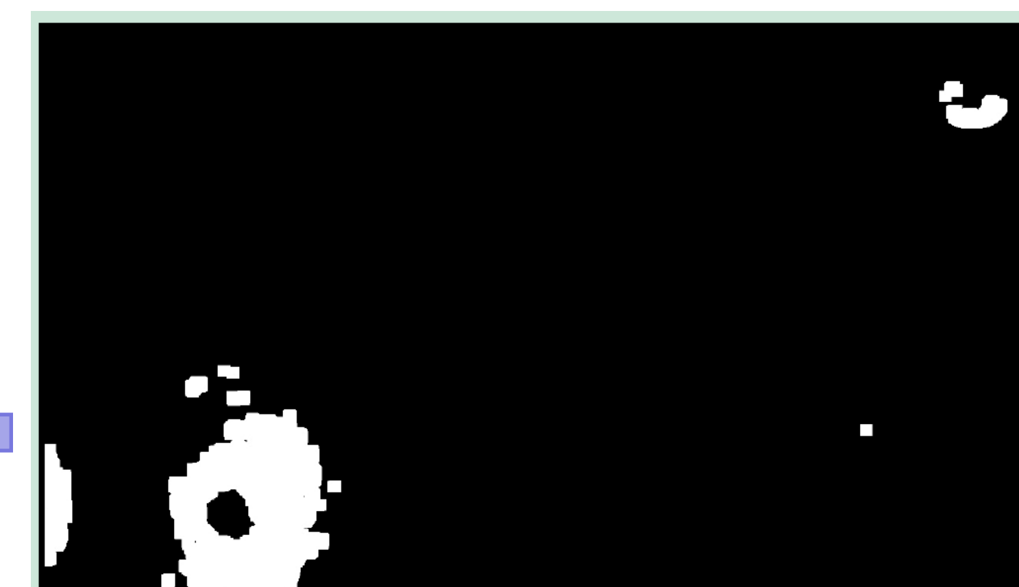
Red Green Chromaticity image after conversion to Hue Saturation Value color space and application of thresholds to find pixels with highest blue values. The resulting image is a binary mask that has underwent one erosion and seven dilations in order to remove high frequency noise and combine fragmented contours.
