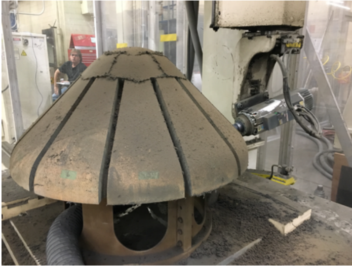
Routing Radial Channels
