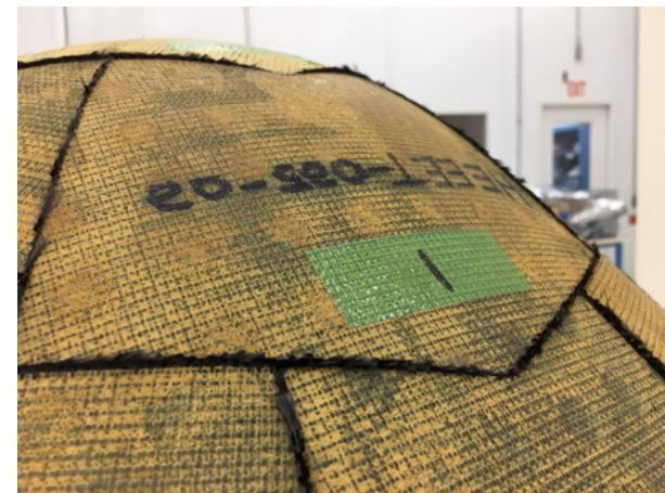
Good OML Match Between Tiles No steps in tile to tile height
