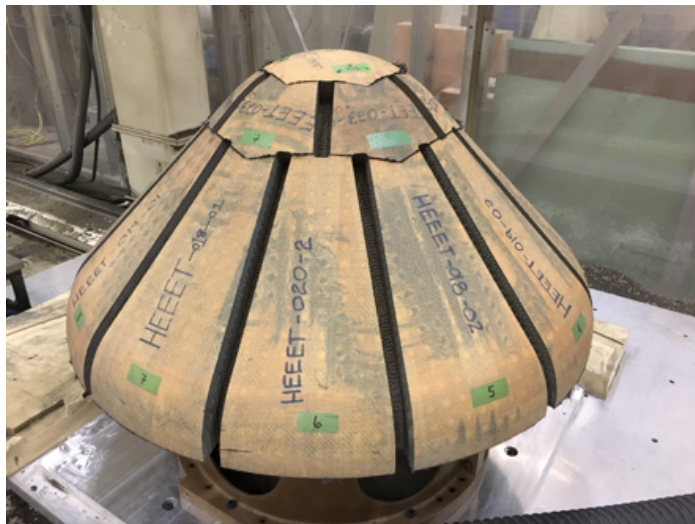
Radial Routing Completed
