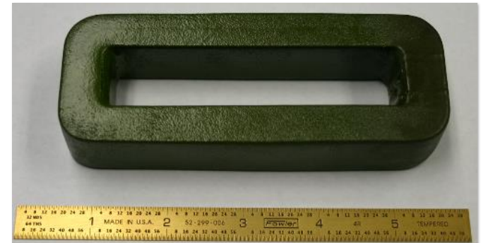
Transformer fabricated from spin cast ribbon
