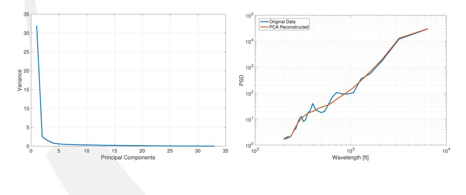
Modify the mean PSD between 200 and 1000 ft wavelengths, by extending the power law fit to the mean PSD for wavelengths between 1000 and 2500 ft
