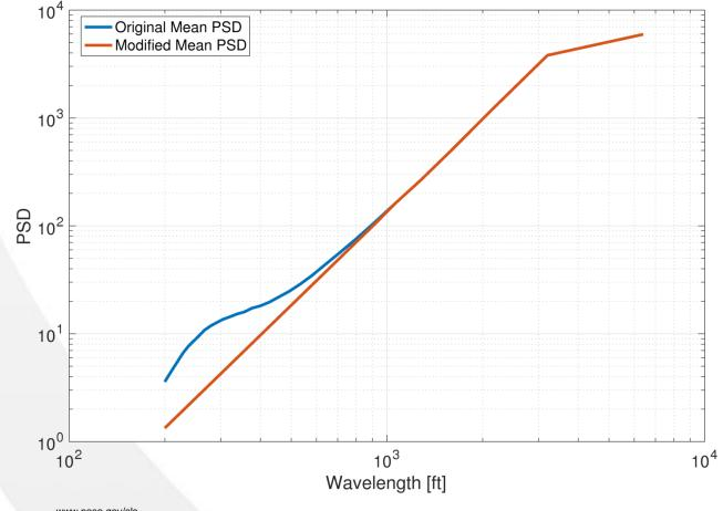
Modify the first 7 principal component shapes (directions) between 200 and 1000 ft wavelengths, by extending the best line fit to the component shape for wavelengths between 1000 and 2500 ft
