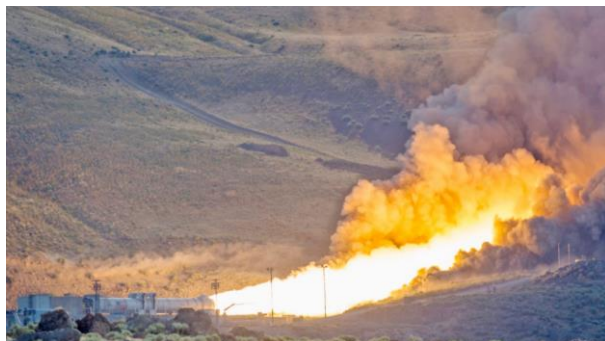
Fig. 6. Qualification Motor-2 test firing.
