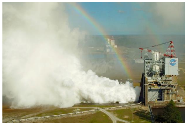
Fig. 8. RS-25 hotfire test at Stennis Space Center.
