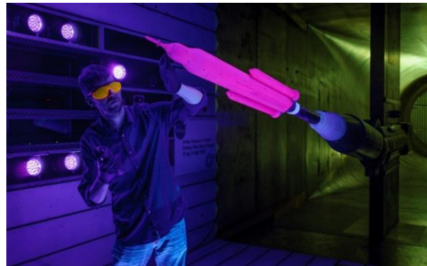
Fig. 11. Block 1B wind tunnel testing at NASA's Ames Research Center.
