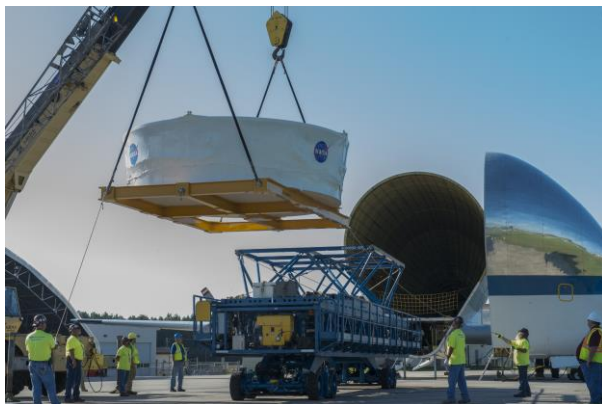
Fig. 10. SLS OSA loaded onto Guppy aircraft.
