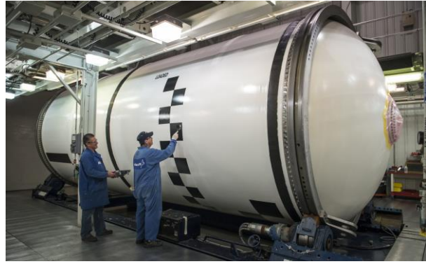
Fig. 7. A completed booster motor segment.
