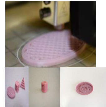
FDM prints using reclaimed anti-static bagging film with reversible cross-linking additive (image from Cornerstone Research Group)
