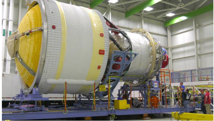
Figure 8 The EM-1 Interim Cryogenic Propulsion Stage, prior to delivery to Kennedy Space Center
