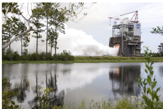
Figure 3 July 2017 test of an RS-25 engine and engine controller unit flight hardware
