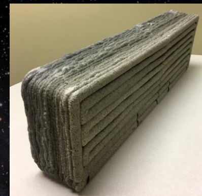
3D-Printed beam (polymer/regolith mix) test specimen from Oregon State University
