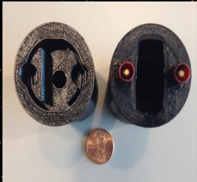
Additively-manufactured fuel grain of ABS. 3-D printed ABS has the unique ability to concentrate minute electrical charges on its surface when subjected to a low energy inductive spark.
