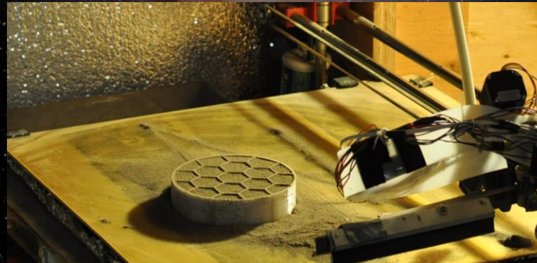
3D-Printing system developed by University of Alaska Fairbanks for the Centennial Challenge
