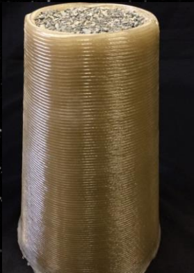
3D-printed compression cylinder made from a polymer and lunar regolith simulant (image from Branch Technologies and Foster + Partners)
