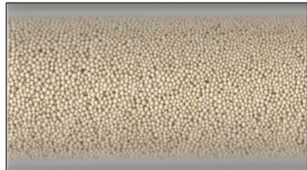
Figure 2.7 Packed (or fixed) bed of zeolite 13X beads. Photo taken by author.
