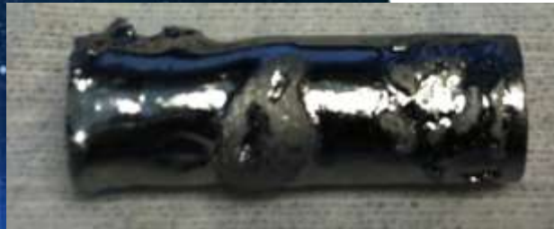
Above/Left: Pure W sample post shakeout run 2. Sample reached melting point (3695K) and was held in place by the BN insulator. BN insulator had to be destroyed to remove the sample
