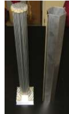
HIP can Mo rod stack up prior to assembly.
