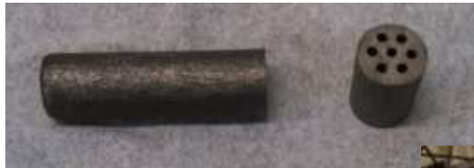
W-ZrO 2 Post Mo etching and HIP can grinding. Sample ready for CFEET testing (Left)
