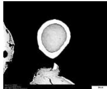
SEM image of W coated ZrO_2
