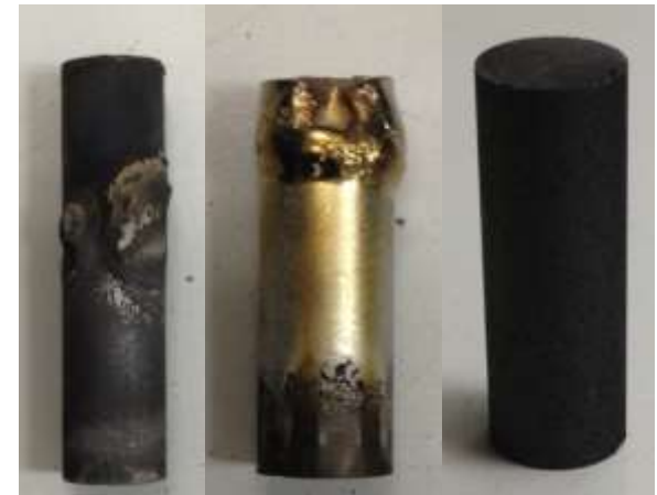
Tungsten, Graphite (L to R) tested in flowing hydrogen
