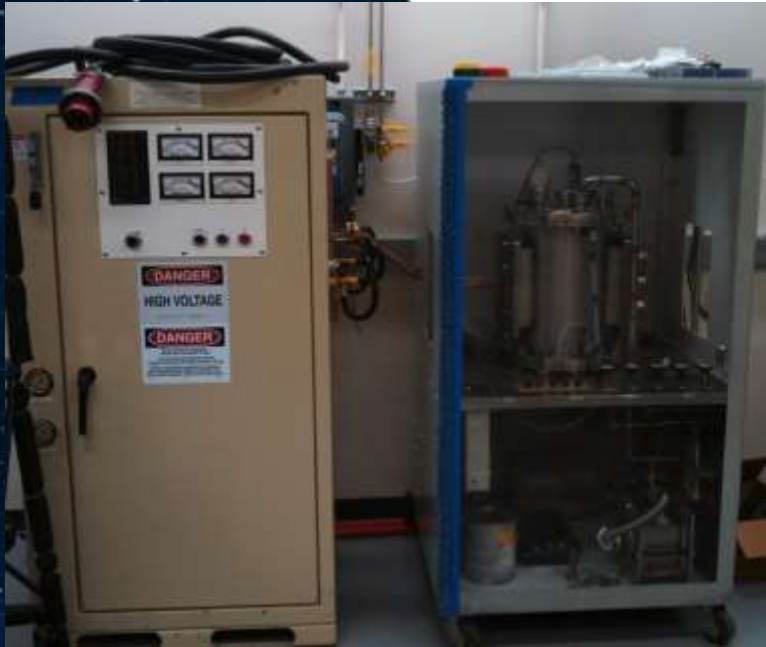
Upgraded CFEET chamber and 50 kW power supply
