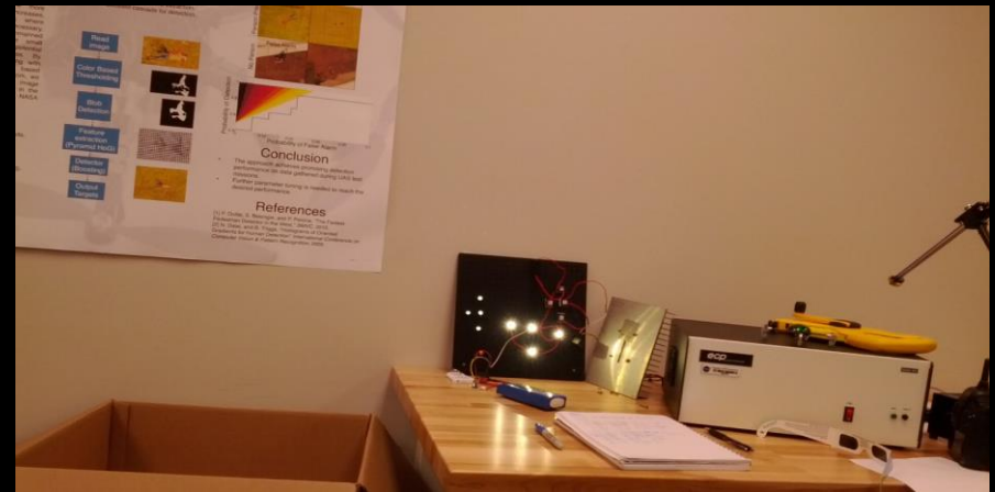
Figure #: Test Setup with LED and retro-reflector targets
