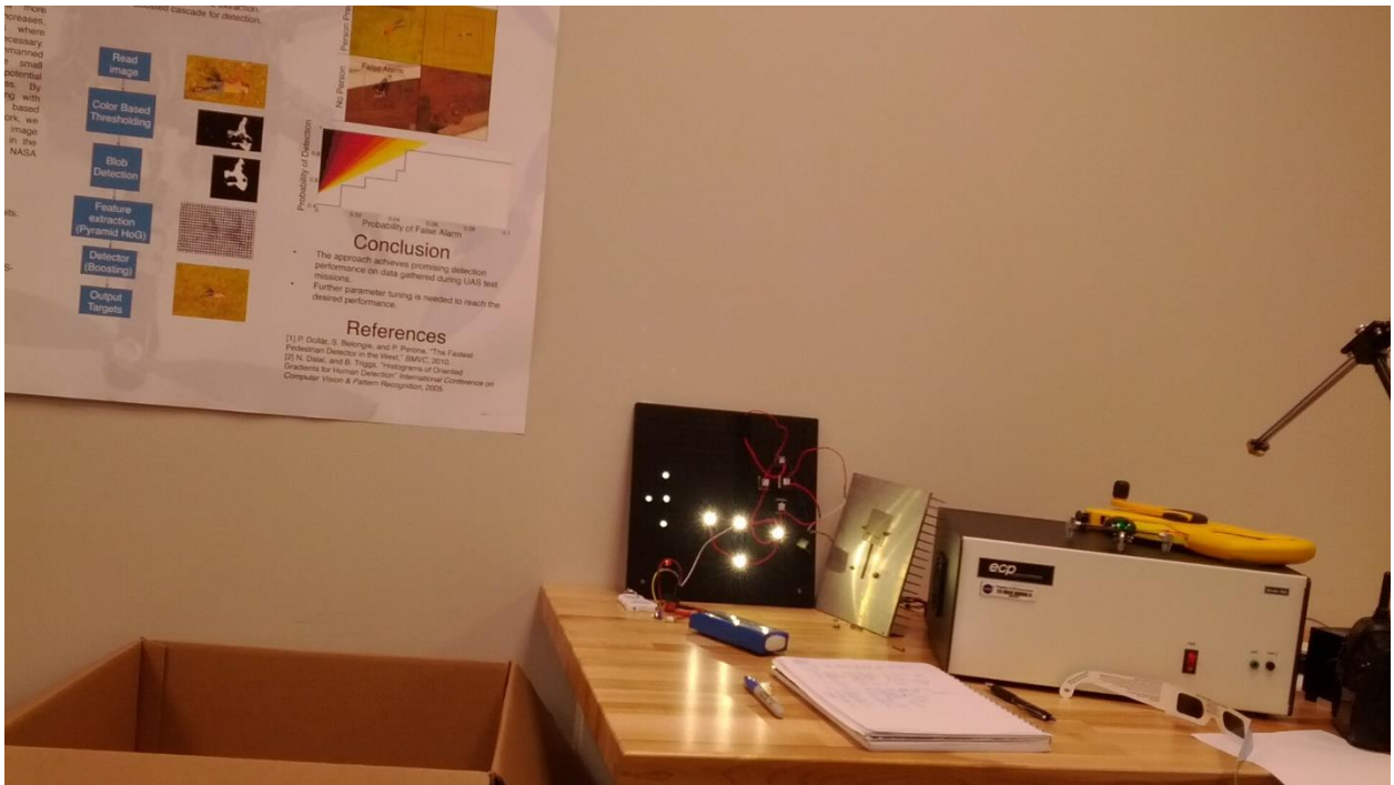
Figure 4. Target Setup for the Comparison Test: Various reflective surfaces were added to the background to test robustness in the face of known false positives.
