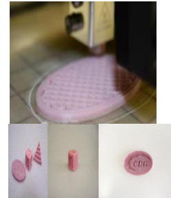
FDM prints using reclaimed anti-static bagging film with reversible cross-linking additive (image from Cornerstone Research Group)
