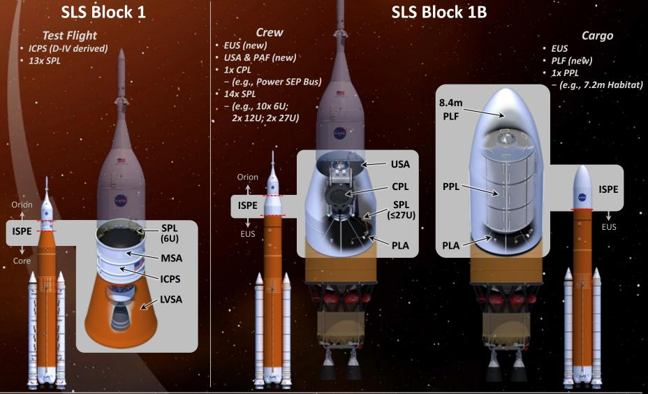
Notes: ISPE – Integrated Spacecraft Payload Element SPL – Secondary Payload MSA– MPCV Stage Adapter ICPS – Integrated Cryogenic Propulsion Stage LVSA – Launch Vehicle Stage Adapter EUS – Exploration Upper Stage USA – Universal Stage Adapter CPL – Co-manifested Payload PLA – Payload Adapter PLF - Payload Fairing PPL – Primary Payload SLS
