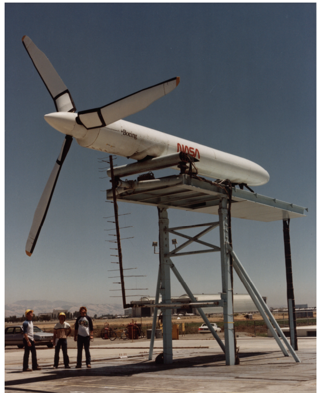
Figure 9. ATB composite-bladed proprotor tested in hover at the NASA OARF.
