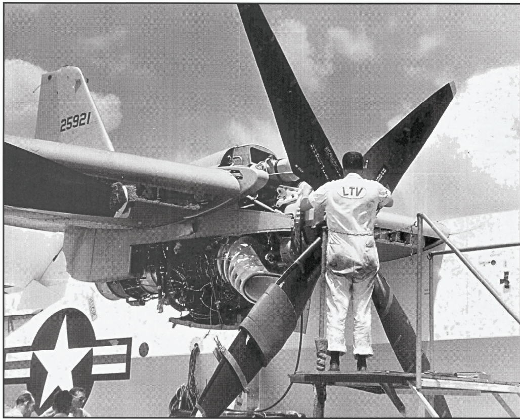
Figure D-1. Initial full-scale propeller (2FE16A3-4A) mounted on the XC-142A.
