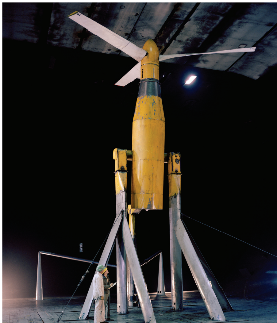
Figure 6. XV-15 metal-bladed proprotor tested in hover in the NASA Ames 40- by 80-Foot Wind Tunnel.
