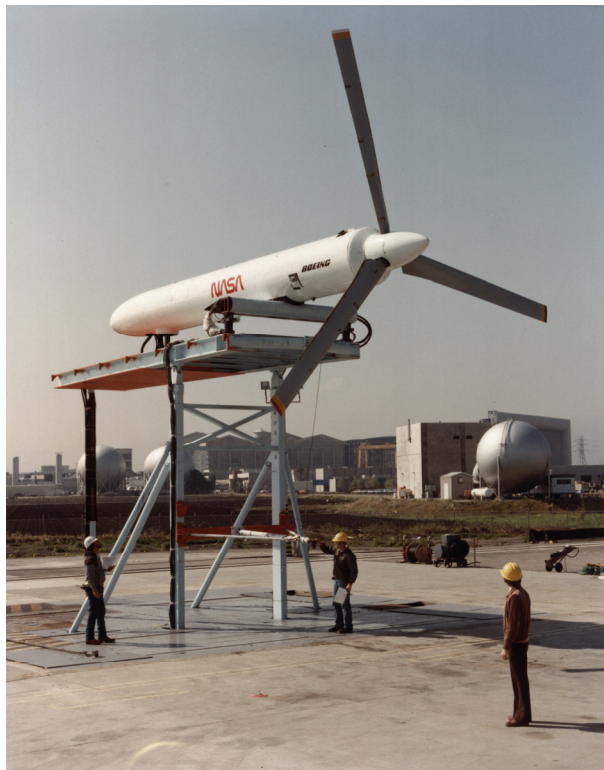
Figure 8. XV-15 metal-bladed proprotor tested in hover at the NASA OARF.
