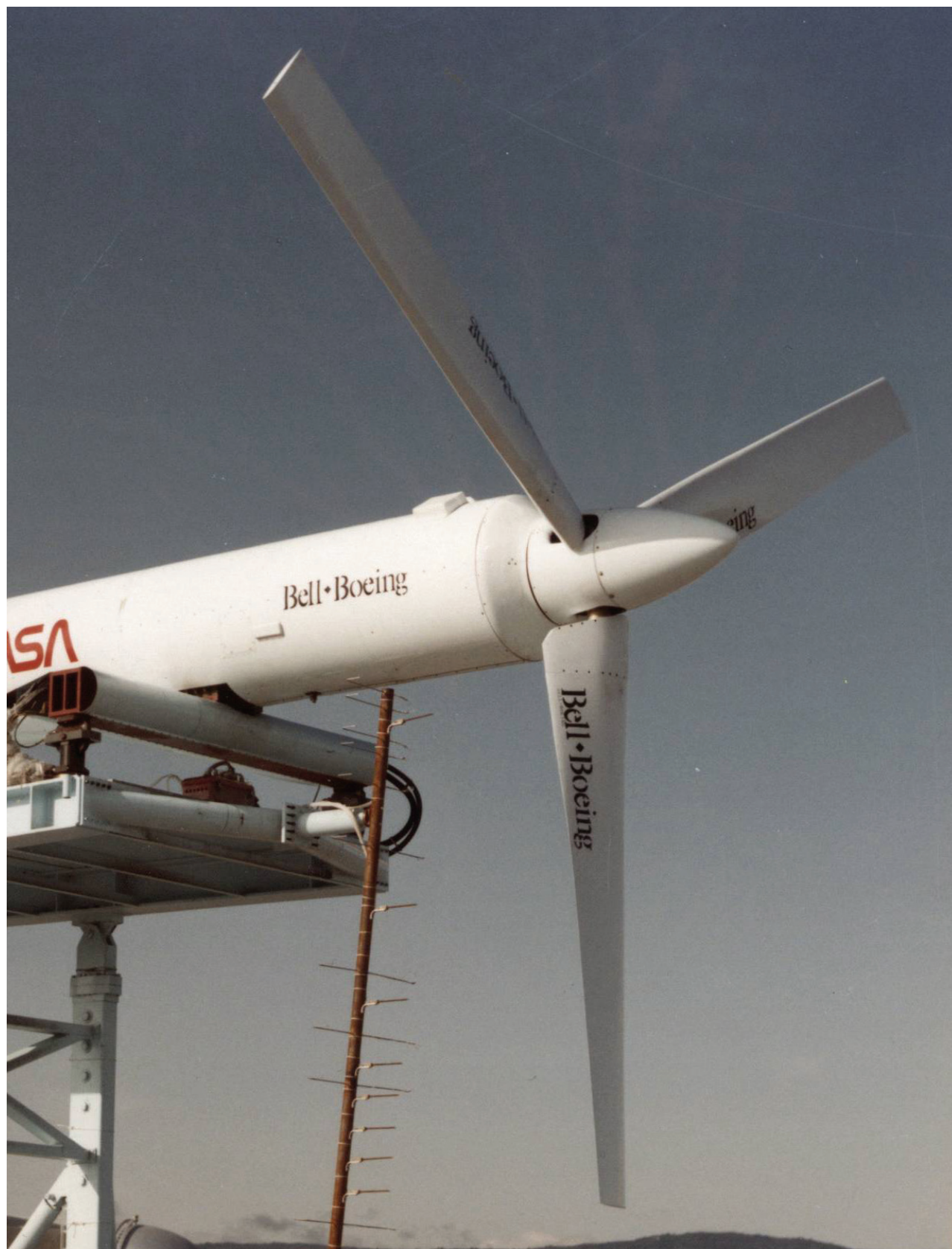
Figure C-1. The 0.658-scale JVX composite-bladed propotor tested in hover at the NASA OARF.
