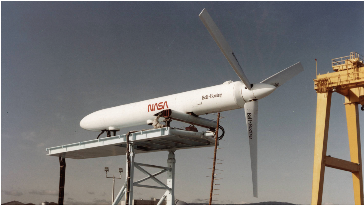
Figure 11. The 0.658-scale JVX composite-bladed proprotor tested in hover at the NASA OARF.
