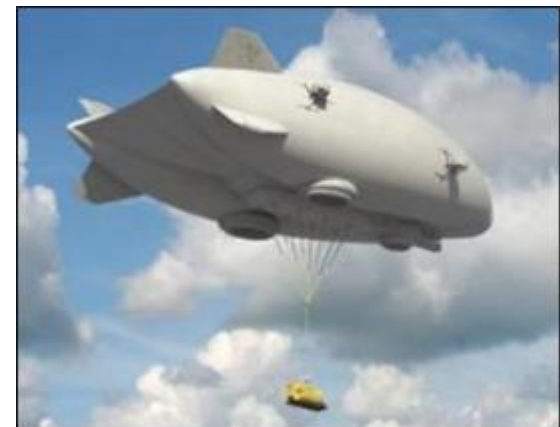
Lockheed Martin hybrid with sling load
