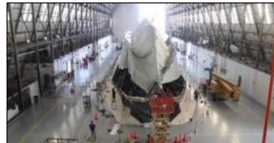
Zeppelin N 07 assembly at Goodyear hangar
