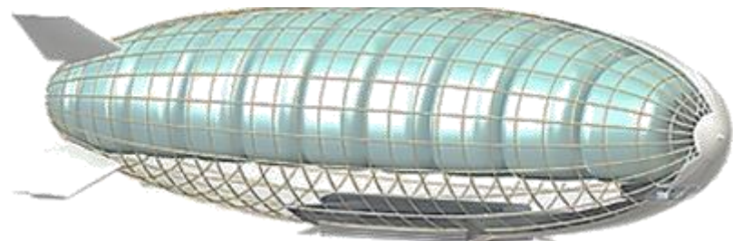
TP Aerospace inflatable rigid hull structural layout
