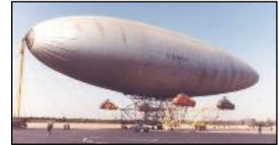
Piasecki Helistat hybrid rotary airship
