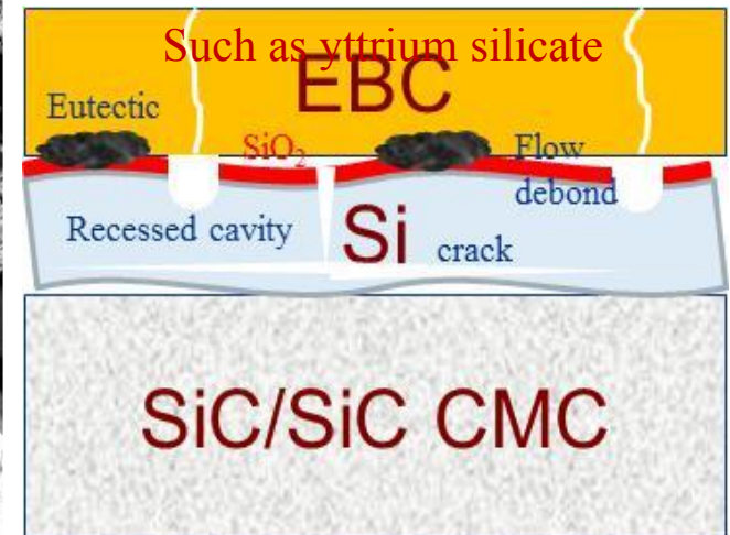
EBC and degradations
