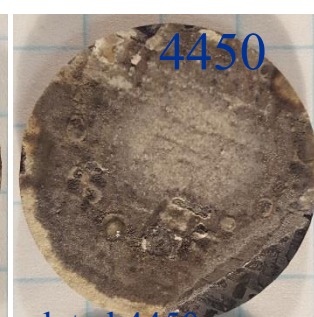
Hybrid Hybrid Zr-rare earth silicate, completed 4450 cycles, 100h
