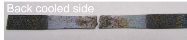
EBC coated CVI-MI CMC with NdYb silicate RESi bond coat, tested T_{surface} 2600^{\circ}F ; T_{back} 2450^{\circ}F
