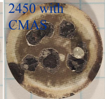
EB-PVD (Yb,Gd,Y)_2Si_2O_7 , total 4450 JETS cycles, 100h
