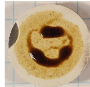
Plasma sprayed (Gd,Y)_2Si_2O_7 , 2450 cycles
