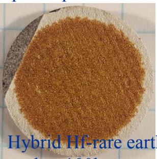
Special processed Yb_2Si_2O_7 , spalling at 450 Cycles
