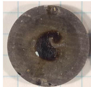
Special processed Yb_2Si_2O_7 , spalling at 450 Cycles
