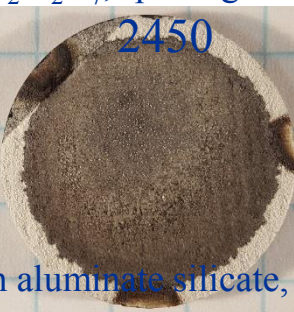
Special processed Yb_2Si_2O_7 , spalling at 450 Cycles
