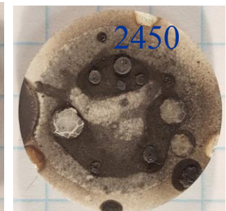
Plasma sprayed (Gd,Y)_2Si_2O_7 , 2450 cycles
