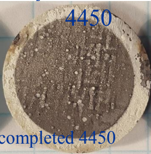
Special processed Yb_2Si_2O_7 , spalling at 450 Cycles
