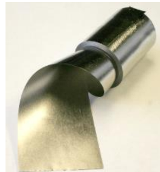
A 25-mm by 1.6-km spin cast ribbon
