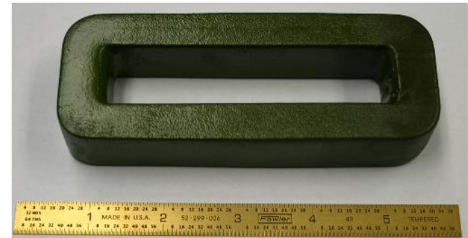
Transformer fabricated from spin cast ribbon
