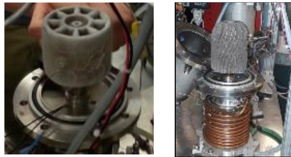
Figure 6. Two possible cold head designs being evaluated for CO 2 collection: (left) 'ferris wheel' design with frozen CO 2 after testing; (right) 'swirl head' mounted in chamber before testing.
