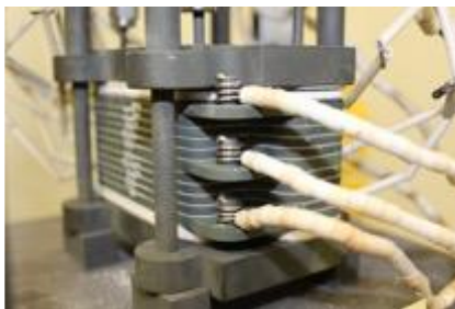
Figure 7a. 10-cell SOE stack built for MOXIE (Ceramatec) in test stand.
