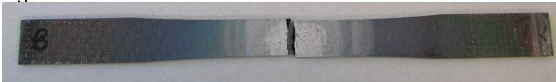
3 hz fatigue testing at 10 ksi loading Completed 500 hr testing
