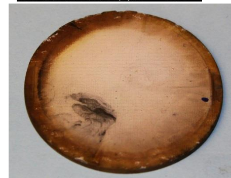
High pressure burner rig, 16 atm, 31 hr
