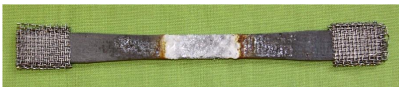
Air Plasma Sprayed APS YSi+Hf-RESi Silicate EBC Bond Coat series on Royce Royce HTC CVI-MI SiC/SiC (with CMAS) 1400°C, at 10 ksi, 400 h
