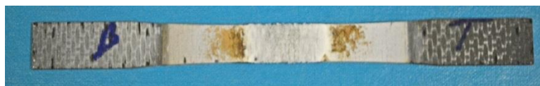
EB-PVD HfRE_2Si_{2-x}O_{7-x} EBC/GdYbSi(O) bond coat on CVI-MI SiC/SiC (with CMAS) 1537°C, 10ksi, 300 h fatigue (3 Hz, R=0.05)
