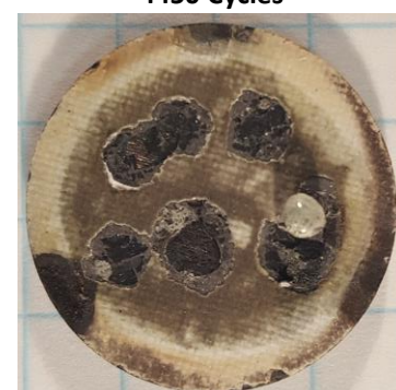
Turbine vane EBC, CMAS JETS tests (100 h)
