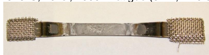
PVD GdYbSi(O) bond coat, 1316°C, 15ksi, 1169 h fatigue (3 Hz, R=0.05) on GE Prepreg SiC/SiC
