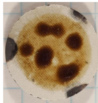
Turbine vane EBC, CMAS JETS tests (100 h)
