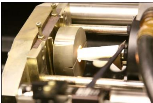
EBC coated Trailing Edge (TE) “wedge” testing in high heat flux and mechanical fatigue loading
