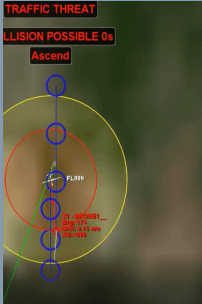
ADS-B DAA Flight 5 - May 2017: Commands Avoidance maneuver to safely avoid the collision
