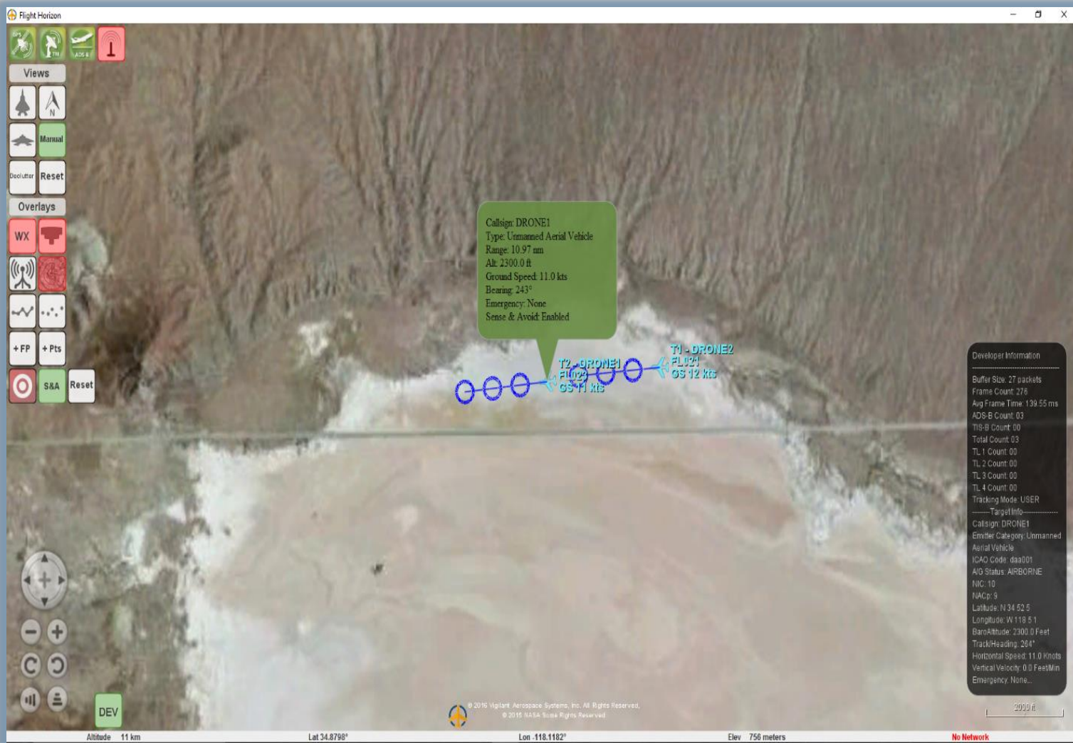
ADS-B DAA Flight 1 - December 6, 2016: Detect and Track intruders using ADS-B
