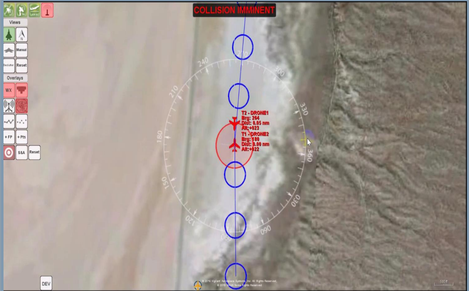
ADS-B DAA Flight 2 - December 7, 2016: Determine if intruder is a collision threat
