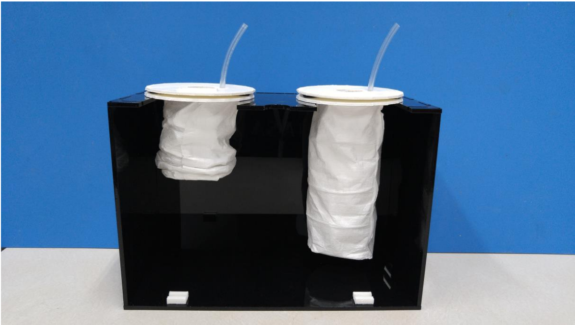
Figure 12. Sealed modules in housing unit. Collapsed module (left) and expanded module (right)
