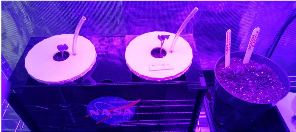
Figure 14. Growth test: top view. Module plants (left) and control plants (right) immediately after transplant
