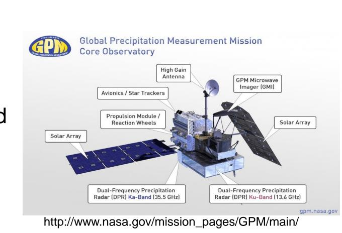
The GPM has a broad global coverage ~70°S – 70°N with a swath of 245/125-km for the Ka (35.5 GHz)/Ku (13.6 GHz) band radar, and 850-km for the 13-channel GMI. GPM also features better retrievals for heavy, moderate, and light rain and snowfall.
