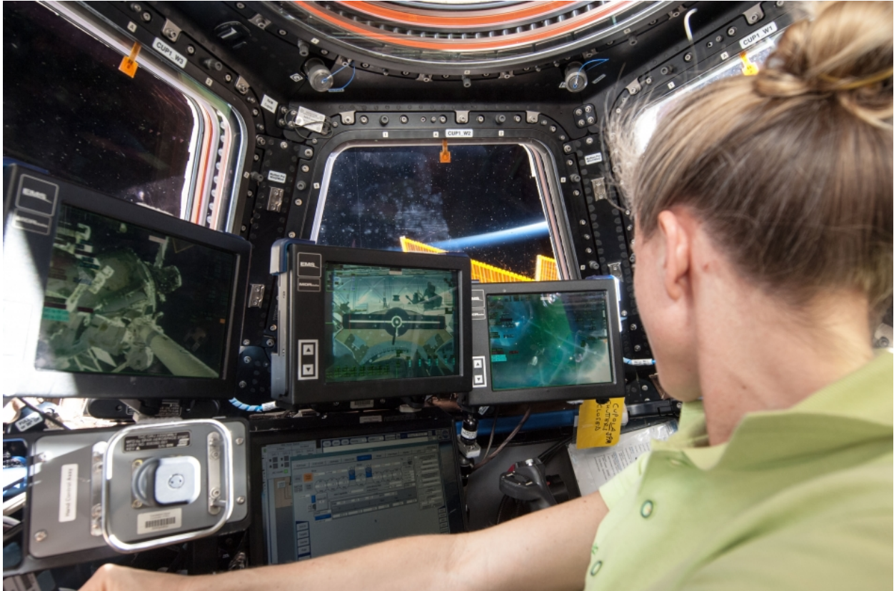
Figure 2: Astronaut Karen Nyberg (Expedition 36) at the robotics workstation in the ISS Cupola preparing for grappling and berthing of the Japanese H2 Transfer Vehicle-4 (HTV-4). Credit: NASA.
