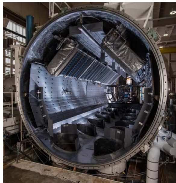
Figure 2. TDU-3 installed in NASA GRC VF-5.
