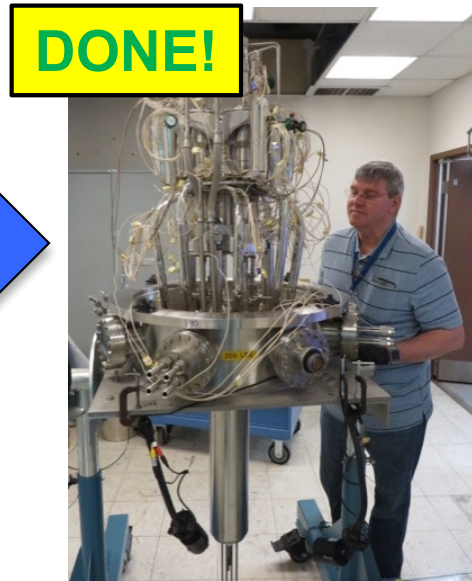
Thermal-Vac System Test with Depleted Uranium (DU) Core at GRC (Phase 2)
