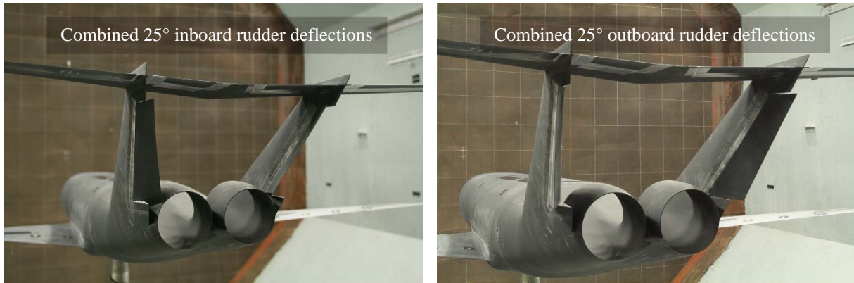
Figure 62 – Pictures of combined 25° inboard and outboard rudder deflections.
