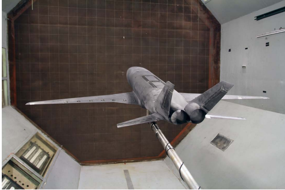
Figure 18 – Aft view of Low-tail configuration in the tunnel.
