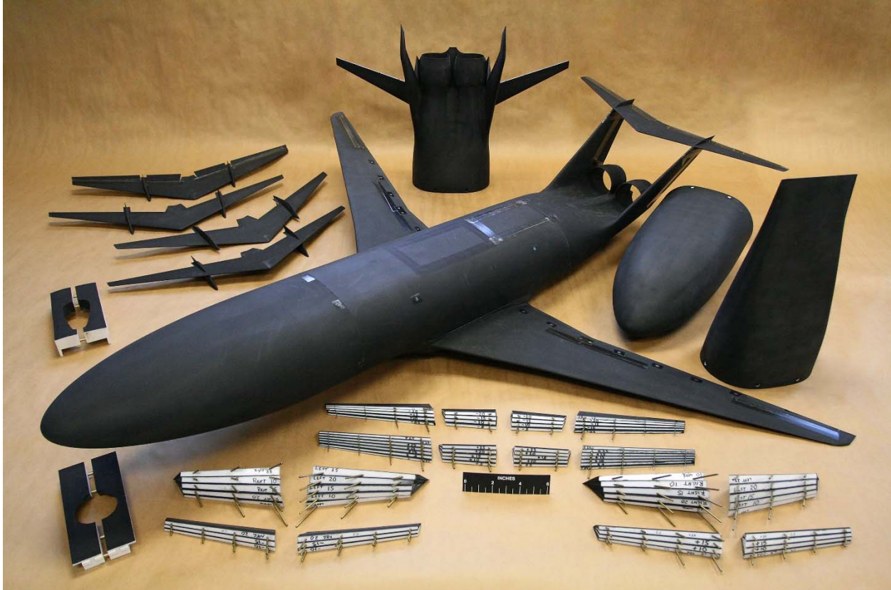
Figure 4 – Five-percent scale D8 model with configuration and control surface parts.
