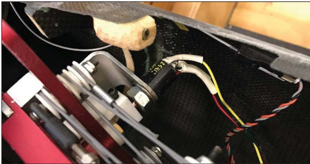
Figure 13. Tail Actuator Arm w/Integrated Potentiometer
