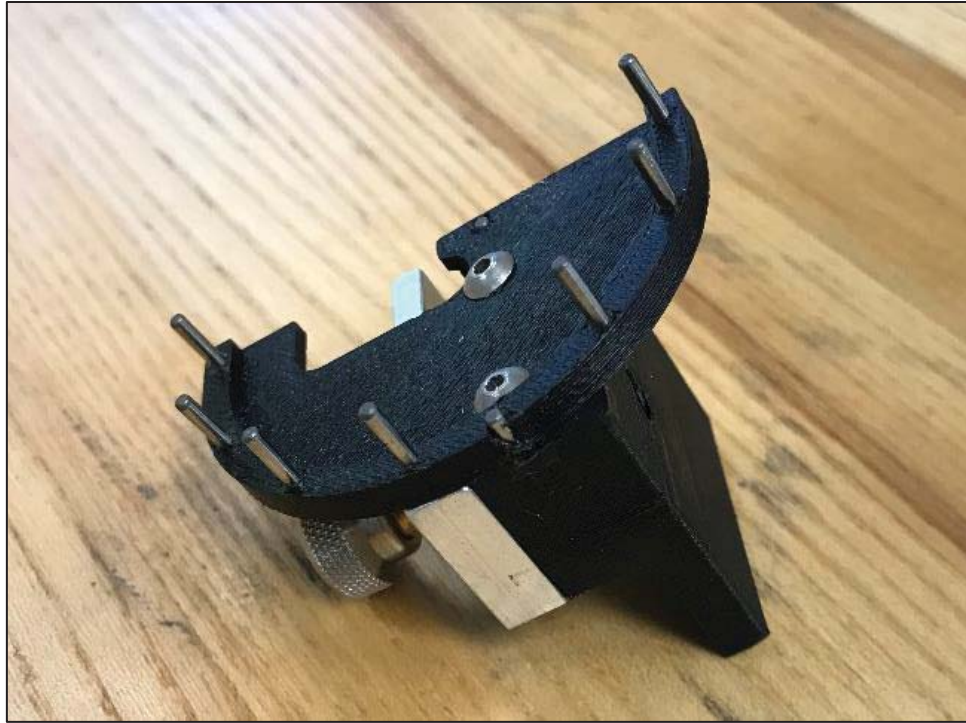
Figure 14. Alpha/Beta Potentiometer Calibration Tool (-30°, 0°, 30°)
