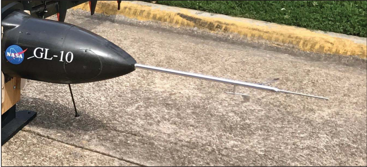
Figure 12. SpaceAge Controls Alpha/Beta Pitot Tube
