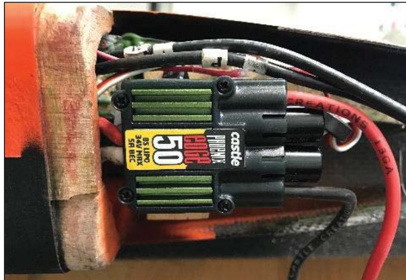
Figure 9. Motor 1 Nacelle w/Integrated ESC
