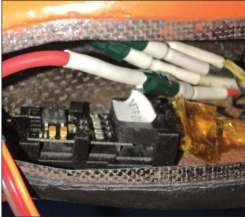
Figure 10. Motor 1 Nacelle w/Integrated Serial Link
