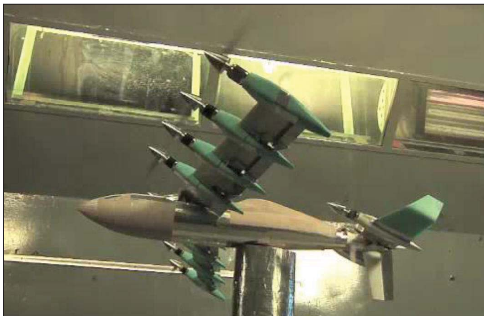
Figure 27. Design of Experiments GL-10 Controls 30% Scale Wind Tunnel Model
