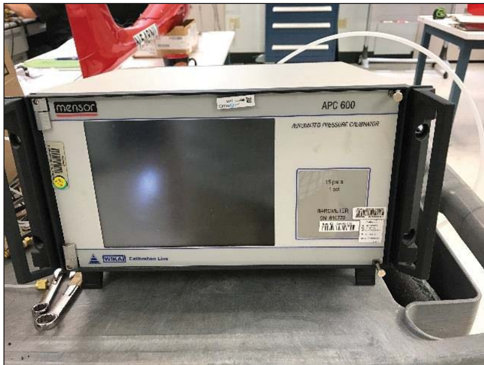
Figure 15. Pitot Probe Calibration Tool (Static/Dynamic)
