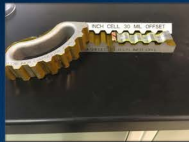
M-SHELLS ribbon cell with in-house designed corrugation tools
